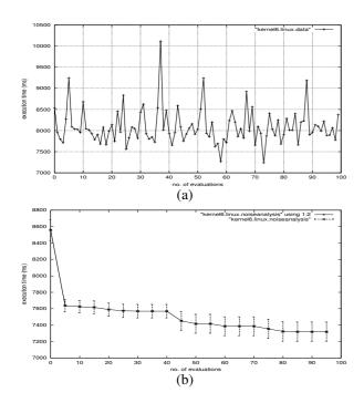
Figure 3. Heuristic search on Linux+Celeron (a) the curve shows the execution time against the number of evaluations during one search on kernel6. It demonstrates the complexity of the optimisation space. (b) the average of the best execution time currently found over 10 searches on kernel6 are plotted against the number of evaluations, as shown in the solid curve. The error bars show that the standard deviations are low, which indicates that all 10 searches achieve very similar results.
